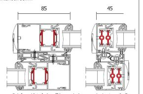
Reinforced interlocks will be used where required automatically
